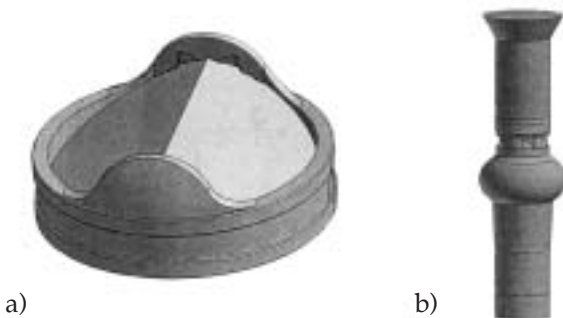
Figure 4: Model geometry. a) 27 mm St. Jude HP valve; b) overall model including the inlet ventricular duct and the outlet aortic duct.
