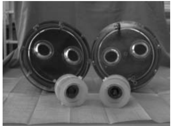
Figure 4: The inner surface of the thrombosis tester after an experiment with non-anticoagulated blood.
