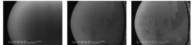
Figure 10: Scanning electron microscopy images of a ZrO_2 inlay run in a PEEK housing. Left: before testing. Center: after 40 million load cycles. Right: after 90 million load cycles.
